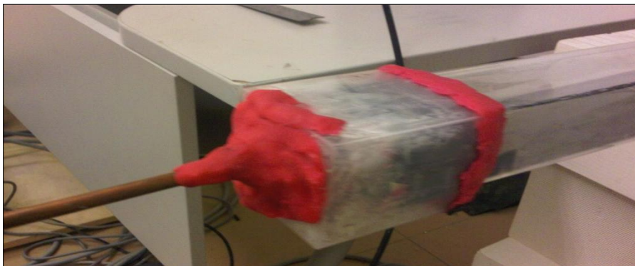
Figure 4.9 The hard end of the quartz resonator showing the plastic box covering the tube end, the seeder output copper tube used to induce seeding particles into the resonator and plasticine (commercial clay) in pink covering the two interfaces of the resonator tube with the plastic box and the seeder tube with the plastic box.
